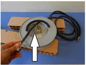
2) Using a 19mm spanner, screw the rubber coupling to the shaft.
