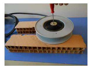
4) Assemble the spring cover and tighten the four M4 screws.
