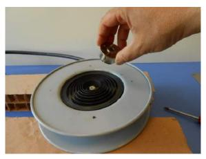
4) Remove the retraction spring.
