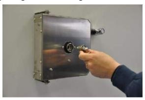
3) Connect the inlet flexible hose to the inlet unit M½"G of the MIDIReeL.
