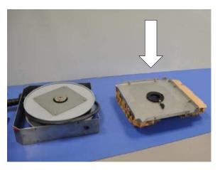
2) Assemble the pulley assembly, the side band and the other shell. Ensure the correct position of the side band in relation to the covers.
