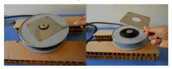
2) Unscrew the central screw inside the central hub.
