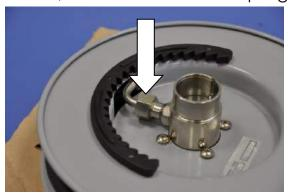
3) Roll the tube onto the pulley and pass the lug over the socket on the side of the MIDIReel.
