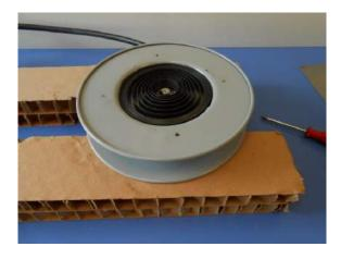
17.2.2. Assembling the retraction spring
