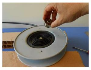
3) Tighten the central screw inside the hub.
