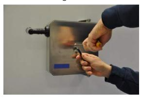
3) Loosen the hub gradually by turning the hex key counterclockwise, to fully unload the spring.
