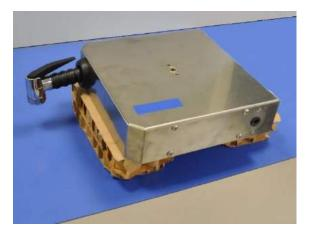
3) Remove the 14 side screws holding the shells together.
